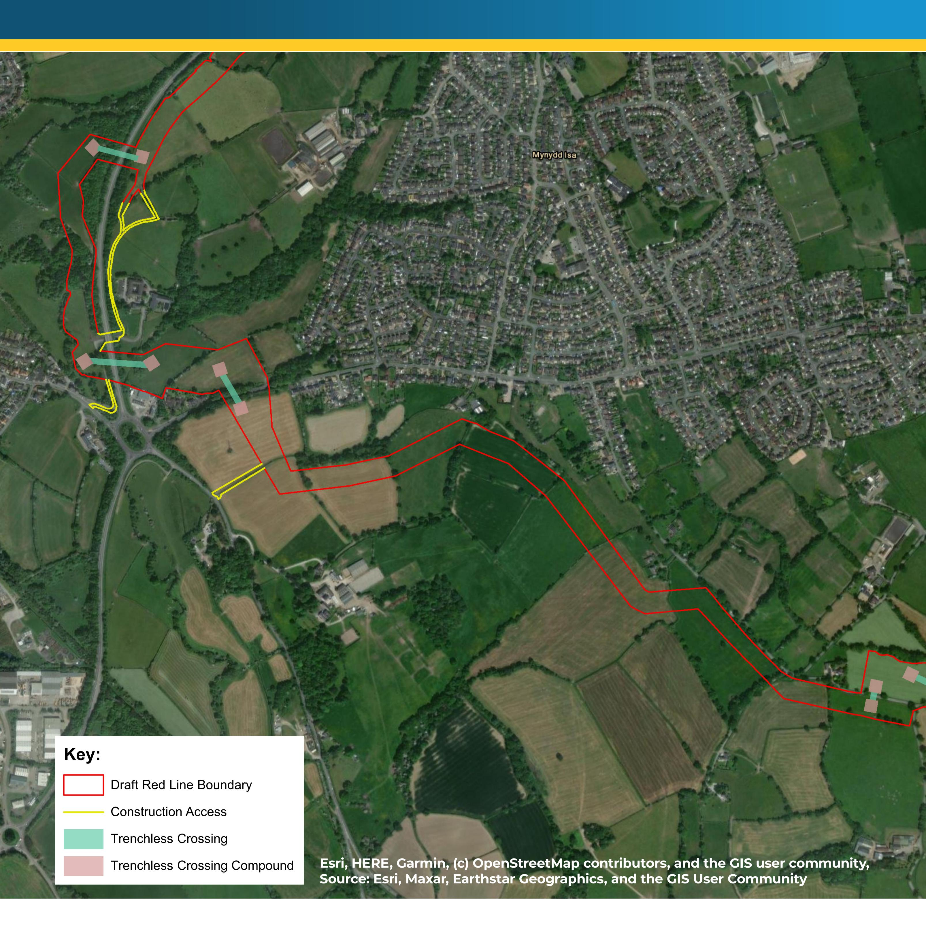
The Padeswood Carbon Dioxide Spur Pipeline route will pass between Mynydd Isa and Mold.
